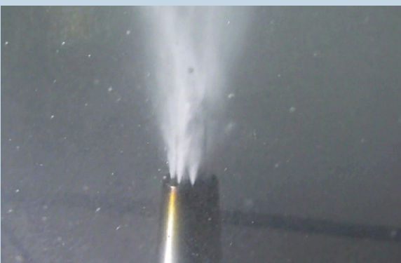
Cool Flash – effektive Kühlung an den Schneiden Cool Flash – effective cooling at the cutting edges
