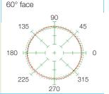
Circularity of center drilled
