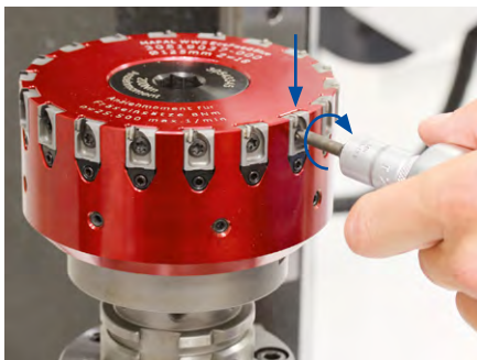
4. Press the milling cartridge lightly while tightening so that the adjusting wedge is in contact. Insert the clamping screw** of the milling cartridge and tighten it clockwise with 1-2 Nm.
