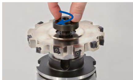
7. Slightly screw the milling cutter clamping screw onto the milling cutter arbor clockwise.
