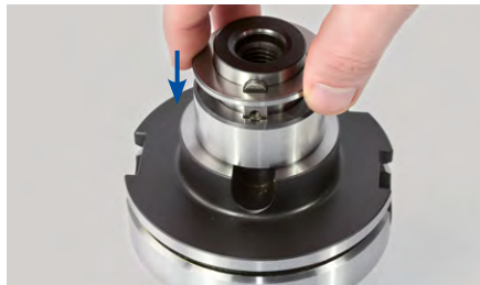
4. Place the second spacer ring on the first spacer ring and the milling cutter arbor.
