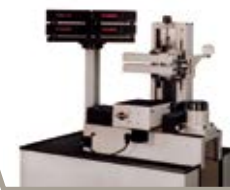
MN 510 The first electronic setting fixture from MAPAL with the vertical arrangement of the tool.
