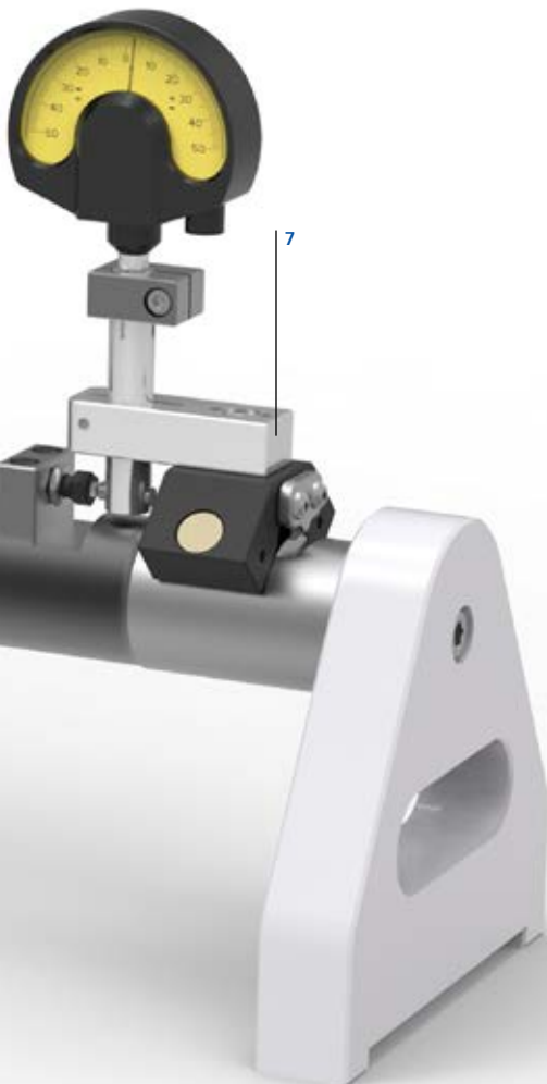
Dial gauge with an accuracy of 1/100 mm.
