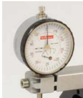
Dial gauge with an accuracy of 1/100 mm.
