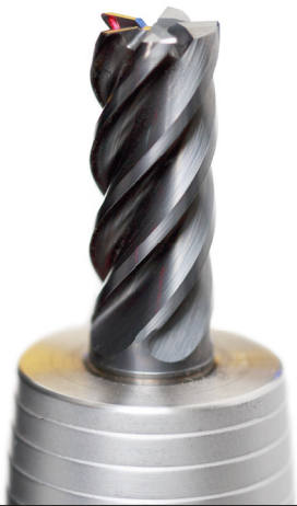
Detail view of a solid carbide end milling cutter with projected laser spot for rough alignment of the measuring position.
