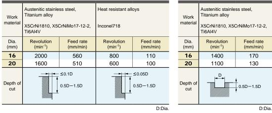
1) If the depth of cut is shallow, the revolution and feed rate can be increased.
