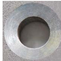
Countersink with extremely unequal spacing
