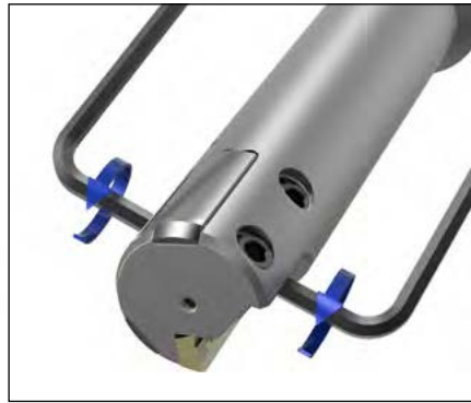
2. Loosen clamping plate: Turn the threaded spindle anticlockwise by 2-3 turns from both sides (insert points downward).
