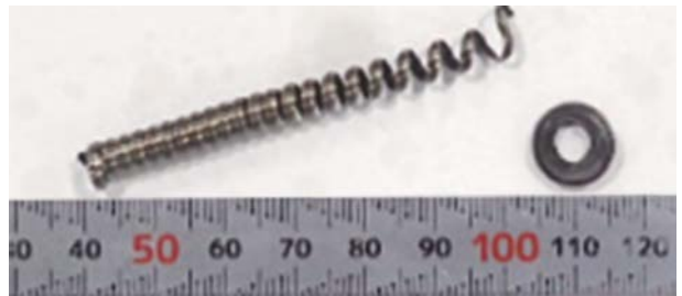
Remaining pip in the centre: \varnothing 0.49 mm, Rz: 0.009 mm
