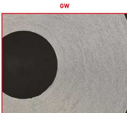
Lead angle 8° – Rz 7.9 μm
