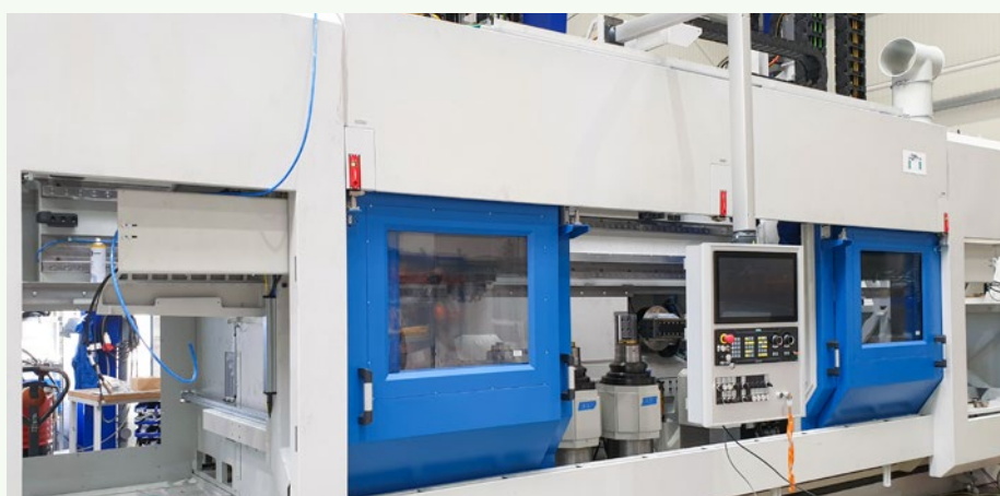
At RASOMA, the next DZS 400-2 is currently being built. The pick-up area is on the left, the drop-down on the right. Various machining stations are set up between them.
