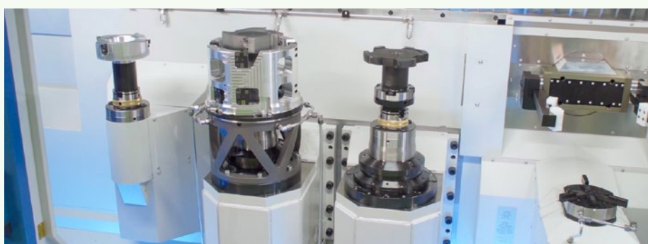
The workpiece is taken to the different machining stations one after the other in the pick-up turning machine.
