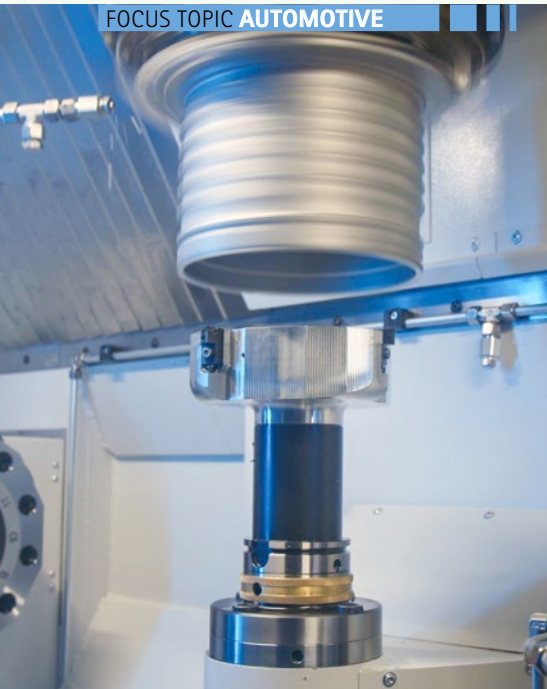
The first step in machining is the pre-roughing of the component's various inner diameters. The tool stands still and only the workpiece rotates.
