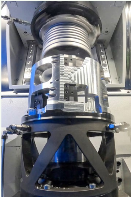
For the second machining step, the thin-walled component is placed in the gap between the inner and outer tool.
