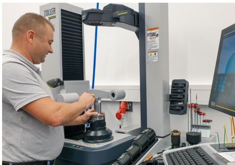
Eugen Bien, application engineer at MAPAL, measuring a NeoMill-Alu-QBig milling cutter.
