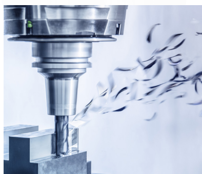
Hybrid Chuck in action: Maximum cutting performance at high tool life
